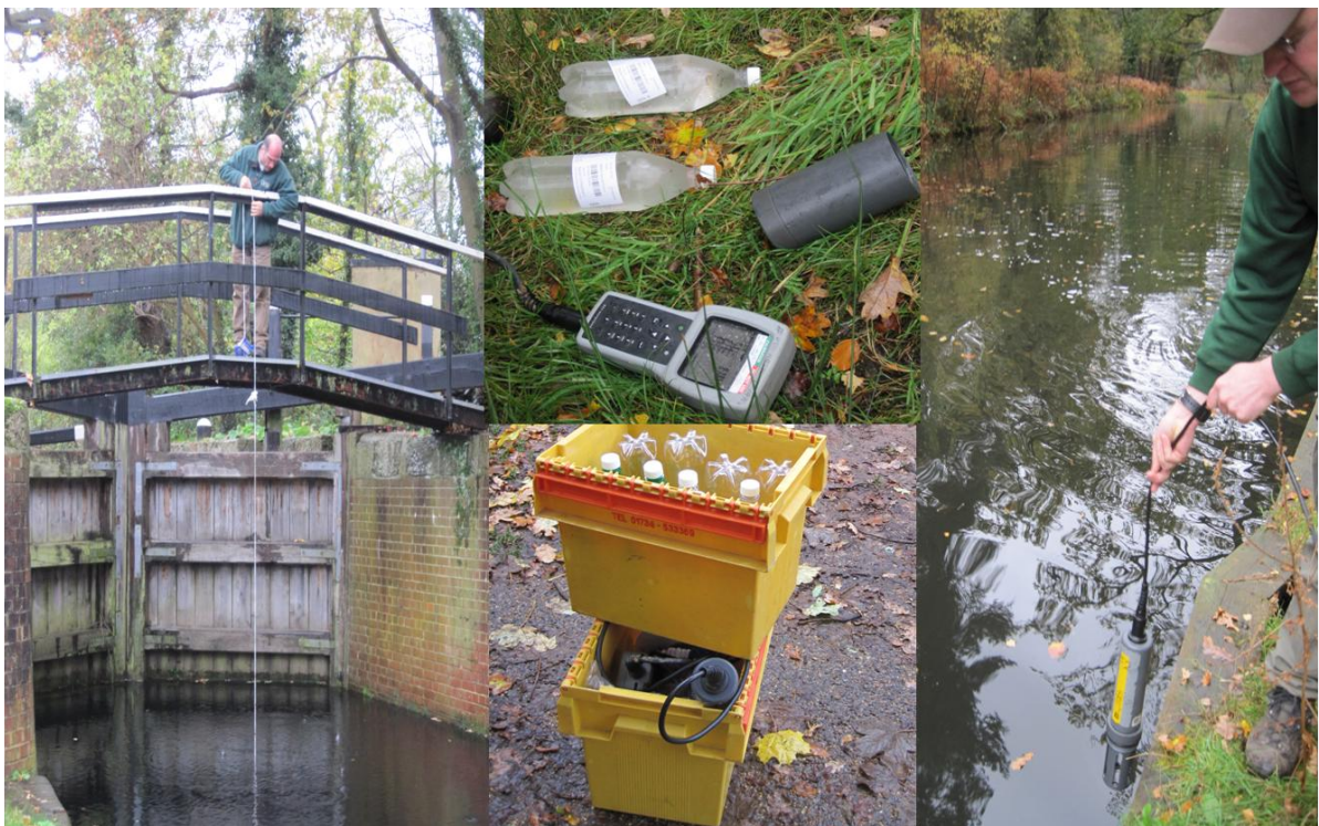
Figure 27 Equipment and processes of water quality measurement
