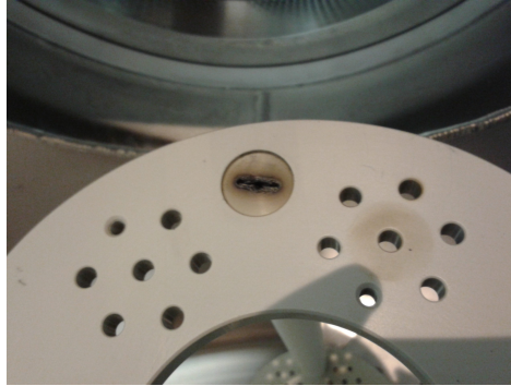
Fig. 3.16: The top of a PEEK screw from the central tripod assembly, which was destroyed during an experiment.
