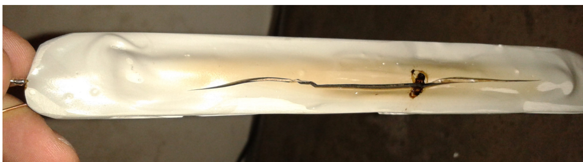
Fig. 3.25: Willow HTE 152 resistor potted in epoxy after an experimental trial. The whole package burst, leading to tremendous outgassing. The approach has been abandoned in favour of several resistors in parallel (see Figure 3.24).
