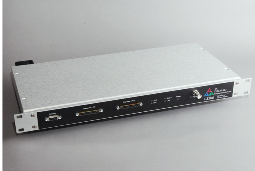
Fig. 4.5: A photo of one of the two 32-channel high precision electrometers used for the current measurements with the wire grid. The electrometer is an off-the-shelf component sold by Pyramid Technical Consultants Ltd.
