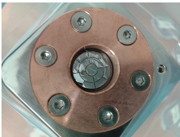
Fig. 5.9: The stripper foil assembly with a 400 atomic layer foil mounted. The round aperture of the grid has proven unfortunate and therefore been abandoned.
