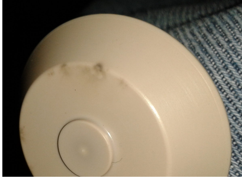
Fig. 3.14: Small traces of carbonisation on insulator surface after high voltage testing of the insulator. The carbonisation happened near the triple point (see also theory in Section 2.6), however this happened to insulators with metallic stress ring as well as to those without. The reason for this is most likely insufficient contact between shell and stress ring.
