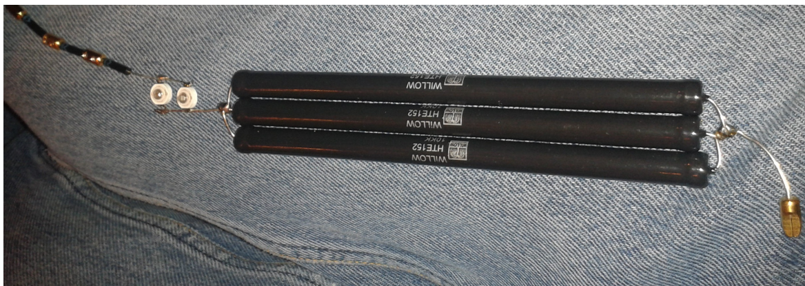
Fig. 3.24: 3 Willow HTE 152 resistors in parallel. They are in series with the high voltage diodes. The chain also contains some LEDs which are used to qualitatively monitor currents going through the diode chain. This resistor setup is very robust and no damage has happened to the resistors in any of our tests.
