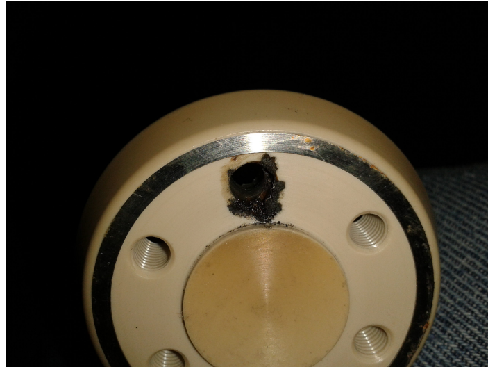
Fig. 3.9: Failure of the insulator with threads. A carbonised path formed through one of the threads.
