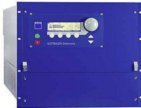
Fig. 2.5: The AC power supply by TRUMPF Hüttinger GmbH + Co. KG. It covers the frequency range of 20 kHz to 100 kHz and has an output power of up to 20 kW. The maximum Peak to Peak output voltage is 2 kV. It uses feedback from its load to determine the resonance frequency.
