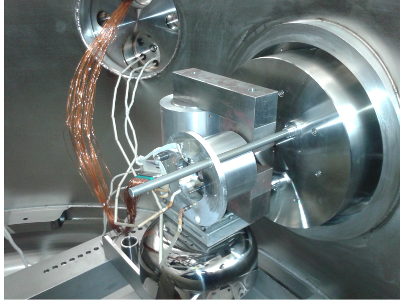
Fig. 4.26: The setup with the dipole magnet between the ion source and the wire grid. The beam deflection of the dipole can be tracked on the grid.
