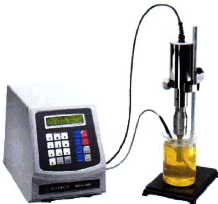
Figure 4 – Model CV 26 ultrasonic processor 1 equipped with a 1.4 cm 2 cross sectional area titanium alloy microtip (Sonics and Materials Inc., Connecticut, USA)
