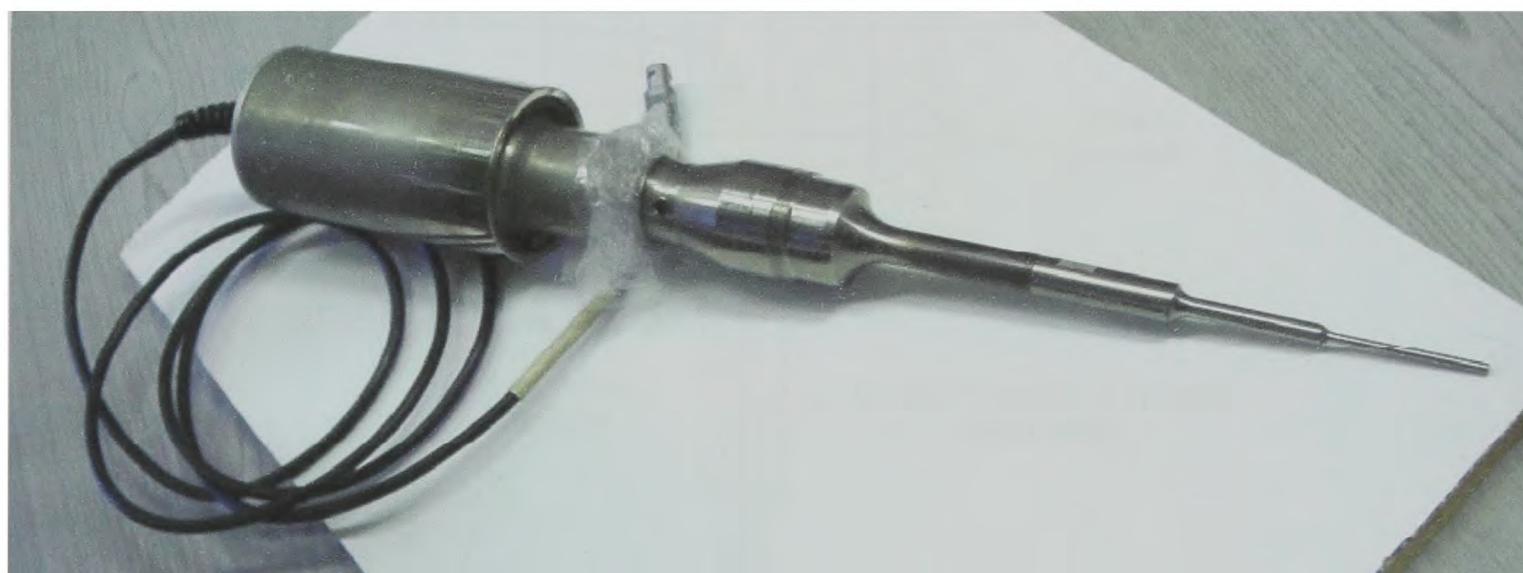
Figure 2 – 20 KHz ultrasonic horn equipped with a titanium alloy microtip of 3 mm diameter
