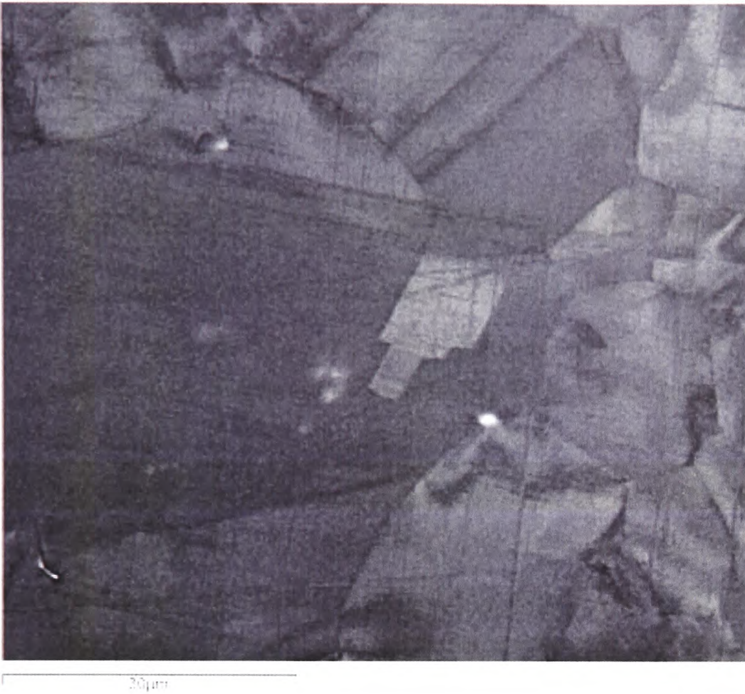
Fig. 3.5. SEM BS picture of a polished x-section of Alloy 600 (acquired in the JSM 6300 in Topo mode).
