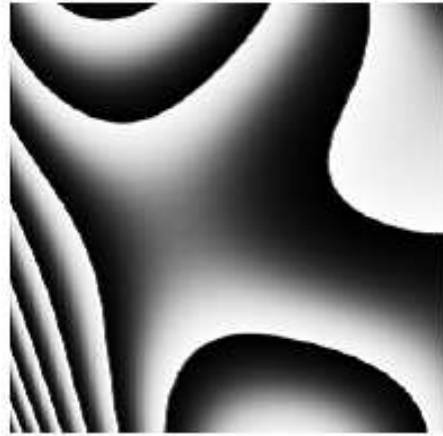
Figure 3.26: Aberration correction result. Zernike coefficients from A_5 to A_{11} are 1.3, 0.11, -0.06, 0.16, 0.11, 0.02, and 0.21.
