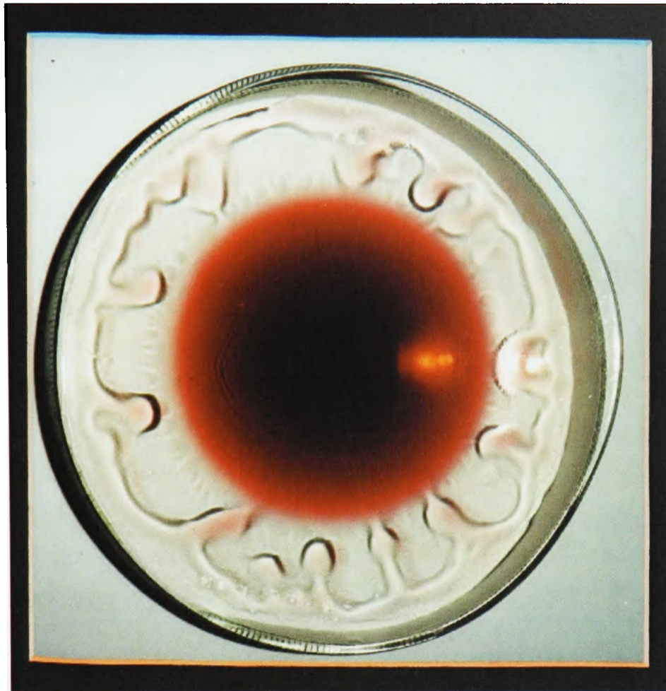
Figure 1.8: Evaporation of alcohol in a wine glass creating a Marangoni stress that causes the wine to climb to the top of the thin film, where it accumulates in a band that grows until becoming gravitationally unstable and releasing the “tears of wine”. Photograph by J.W.M. Bush, Fluid Dynamics Group, MIT, Cambridge, Massachusetts, USA [76].
