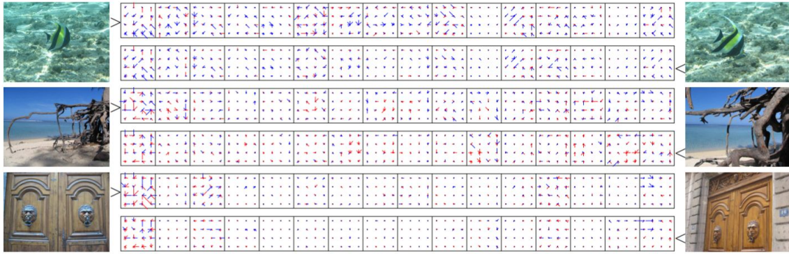
Figure 2.3: Images and corresponding VLAD descriptors (with K=16 centroids). The components of the descriptor are represented like SIFT, with negative components in red. Each box shows a residual of each cluster. Image taken from (Jégou et al. (2010)).
