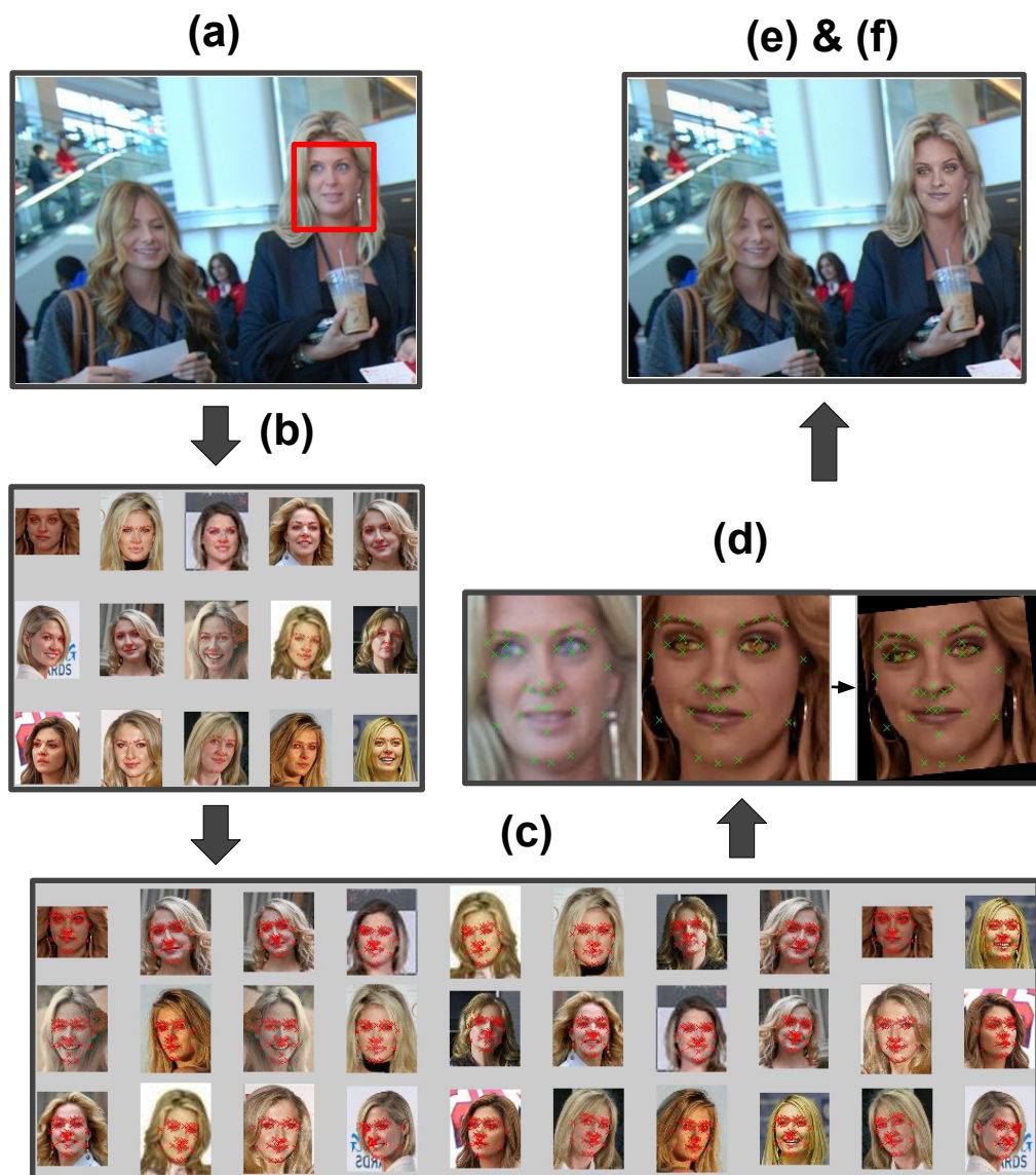
Figure 4.1: Automatic synthetic rendering pipeline. Replacing the face of the unknown person in the airport with the celebrity face (Gage Golightly). (a) Face detection and 36 landmark points annotation on the target image. (b) Top K most similar images (based on FC7 feature vectors) in the face source dataset. (c) Pose descriptors are computed based on face landmarks for these top K images and their flipped version. Top N images in the re-ranked list based on pose similarity are qualified as source faces for replacement. (d) During face replacement, a similarity transformation is computed between corresponding landmark points to map the source face onto the target one. (e) Poisson Editing is applied to produce natural-looking synthetic images. At this stage, the original face is replaced by the labelled source face in the image. (f) As a quality control, the synthesized image is passed to the Face CNN and retained only if the new face can still be recognized.
