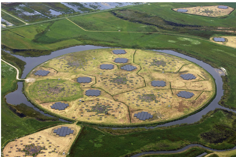
(b) The “Superterp” of the Low Frequency Array, which operates between 10MHz and 240MHz. This photo shows only a fraction of the total telescope, with the circular Superterp island itself covering a diameter of \sim 250 m. LOFAR currently comprises an international network of 54 sub-arrays, with signals combined from more than 5,000 individual antennas. Photo reproduced from van Haarlem et al. (2013).
