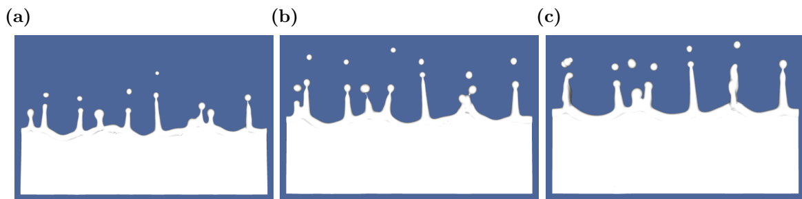
Figure 6.12: Snapshots taken from a simulation case at We = 160 , \varepsilon = 0.04 and N_{\max} = 25 showing ligaments merging on the corrugated rim bordering the expanding sheet, while shedding fragments via the end-pinching mechanism. From left to right: t/\tau_{\text{cap}} = 0.73 , 1.09 and 1.45.
