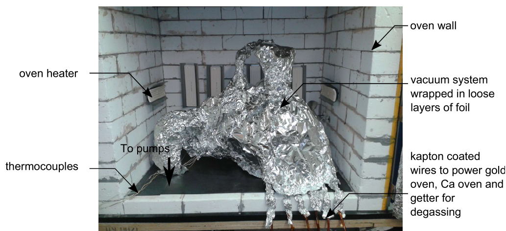
Figure 3.19: vacuum system in the oven, ready for the soft bake. Many loose layers of aluminium foil are used ensure that the heat permeates the system slowly, without creating large temperature gradients which could damage viewports or crack delicate ceramic feedthroughs.
