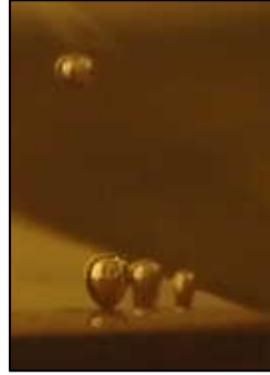
Figure 14: Bubble nucleation process and departure diameter at the onset of nucleate boiling on flat surface, showing attached and growing, departing, and departed bubbles.
