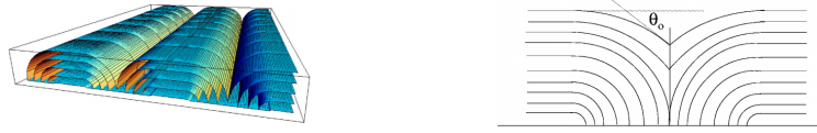
Figure 1.2: Schematic illustration of flattened hemicylinders (left) and curvature wall (right) in smectic-A thin films. Source: [Mic+04, Fig. 9 & Fig. 16].
