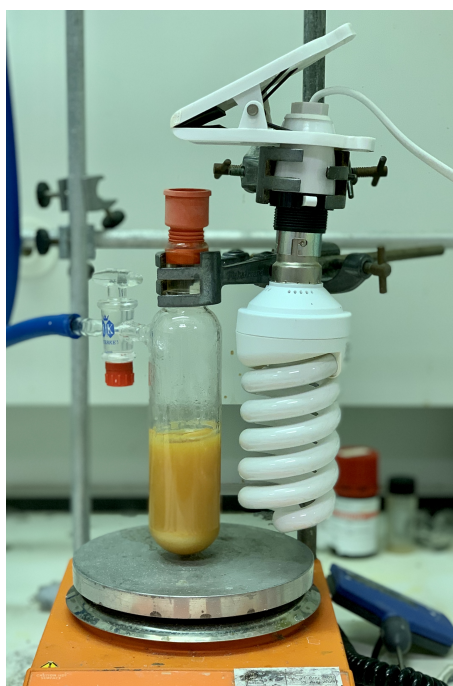
Reaction set-up for the cyclisation of indole 11 on 1.0 g scale (3.6 mmol).
