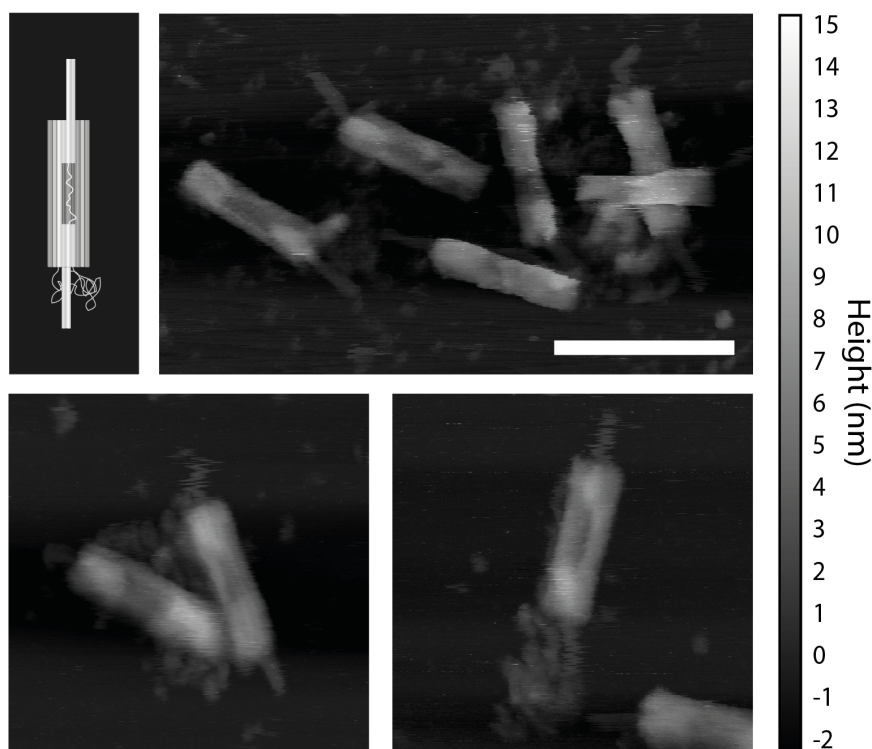
Figure 3.8: AFM images acquired of tightrope origami with 102 nt across the 35 nm gap with 200 bp dsDNA loops either side. Top left shows design schematic for comparison. Scale bars 100 nm.
