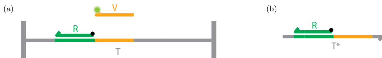
Figure 4.6: Hybridization experiment schematic. a Schematic of the single-stranded tightrope segment bearing quencher probe R . Hybridizing probe strand V is able to hybridize to its complement domain immediately adjacent to R which holds the Cy3 fluorophore close to the Iowa Black FQ quencher on R , reducing fluorescence intensity upon hybridization. b Normalisation complex is able to form 22 bp with V to achieve a ‘fully quenched’ fluorescence level.
