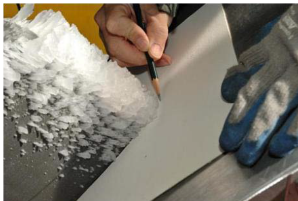
Figure 2.17: Cross-sectional ice shape tracing method. Section of ice is melted and accretion edge traced on a piece of card [78].
