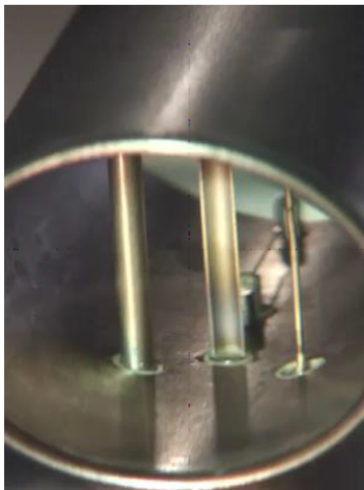
Figure 2.16: Multi-wire liquid water content probe. The sensing elements of the Multi-wire, are the 2.1-mm hollow cylinder (left), the 2.1-mm diameter forward facing half-pipe (centre), the 0.5-mm wire (right), and the compensation wire (behind). [73].
