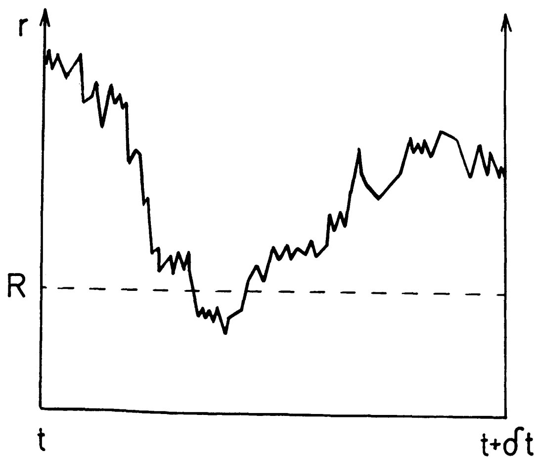
Fig.II.2.2 Encounter during a time step. A schematic representation of the variation in interparticle separation. Reaction occurs when r \leq R .
