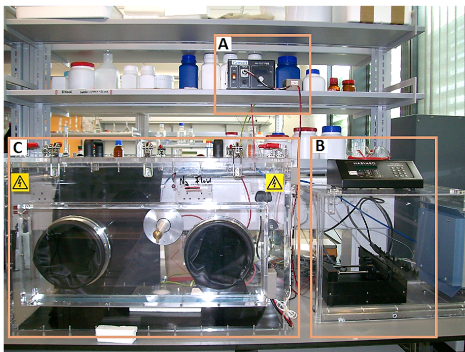
Figure 3.1: Electrospinning setup showing the HV power supplier (A), the syringe pump (B), and the glove box where the fibre meshes are produced (C).
