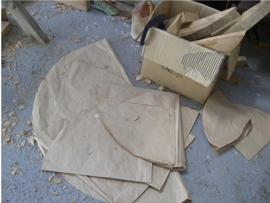
Kraft paper templates used in fabricating cross sections of the sphere at decreasing intervals of 2 inches. The master template was sealed inside the sculpture at completion.
