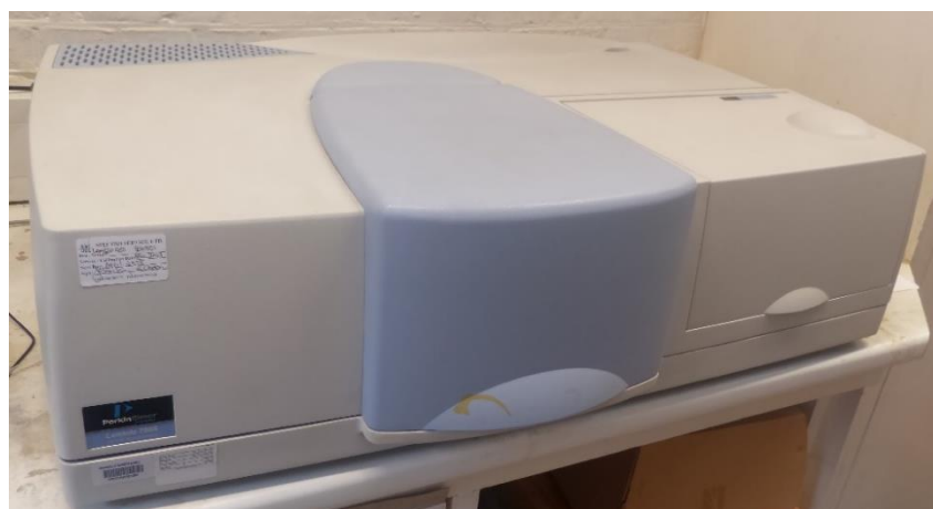
Figure 3-3. The Perkin-Elmer LAMBDA 750S UV/Vis/NIR spectrometer in Inorganic Chemistry Laboratory building (Department of Chemistry, University of Oxford).
