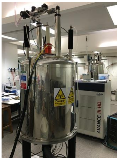
Figure 3-6. The Bruker AVIII 400 (solids) NMR spectrometer in Chemistry Research Laboratory building (Department of Chemistry, University of Oxford).
