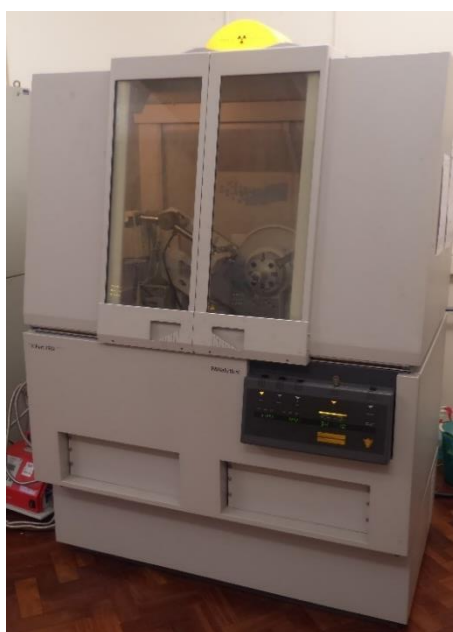
Figure 3-2. The PANalytical X'Pert Pro X-ray diffractometer in Inorganic Chemistry Laboratory building (Department of Chemistry, University of Oxford).
