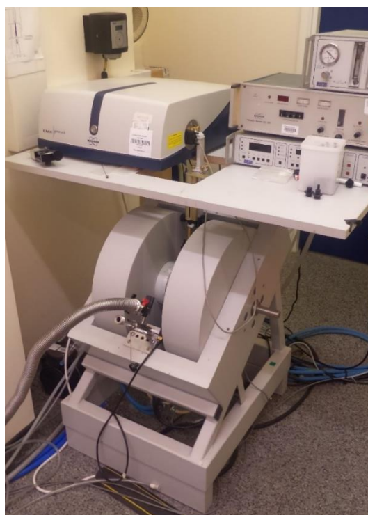
Figure 3-4. The X-band CW EPR spectrometer in Inorganic Chemistry Laboratory building (Department of Chemistry, University of Oxford).
