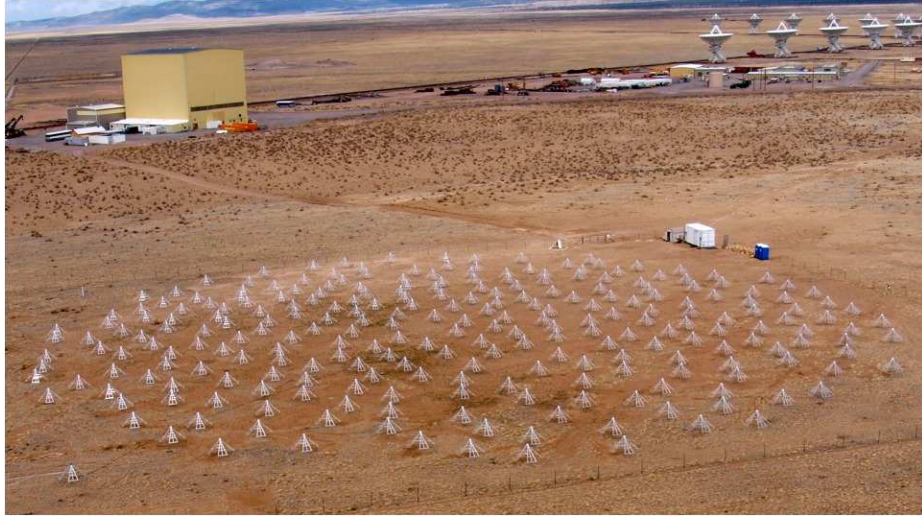
Figure 1.9: A station of the Long Wavelength Array (LWA) array, located in New Mexico. 256 antennas are visible in the core plus 1 outrigger antenna. The antennas have a dual-polarization design with low-noise amplifiers mounted on the top. Signals are routed underground to the correlator in the white cabin next to the array. The site is in close proximity to the VLA, which is visible in the upper right. (Image from phys.unm.edu ).
