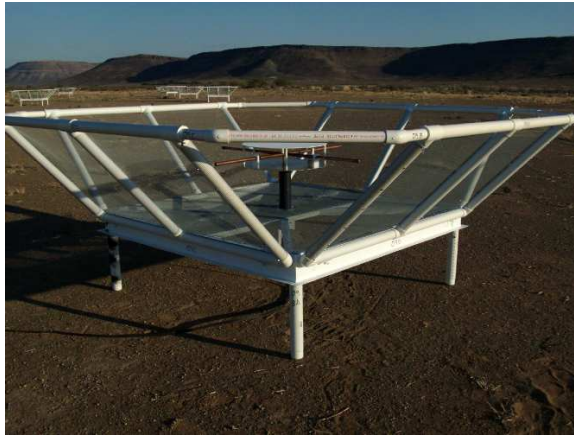
Figure 1.8: PAPER dipole antenna. The copper dipole is surrounded by a ground screen with side panels made of steel and wire mesh, which narrows the antenna’s beam size to approximately the size of cold patches in the synchrotron sky [75]. (Image from eor.berkeley.edu ).
