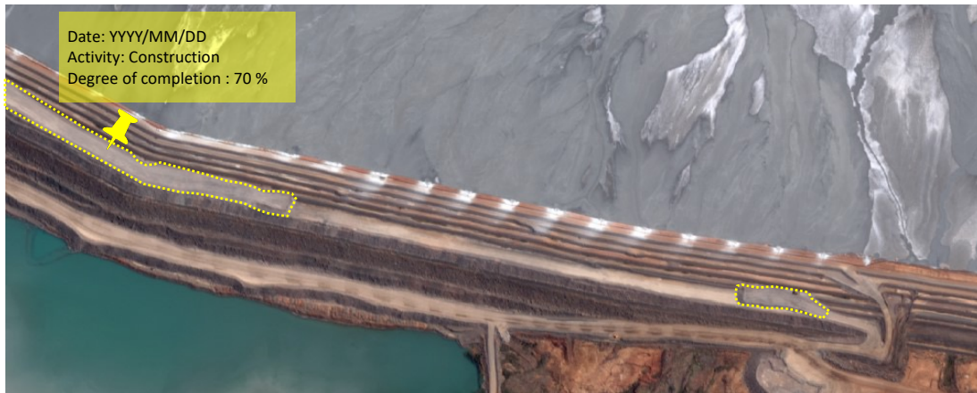
FIGURE 7.1: A mock up of EO data based verification and labelling of construction activities on the ground. Static FE model is not representative of the dynamic state of a TSF. Therefore, the satellite data can help inform the completion status, therefore, the various stress states at different parts of the TSF through time. Imagery © MAXAR and modified from Thomas et al. (2019).
