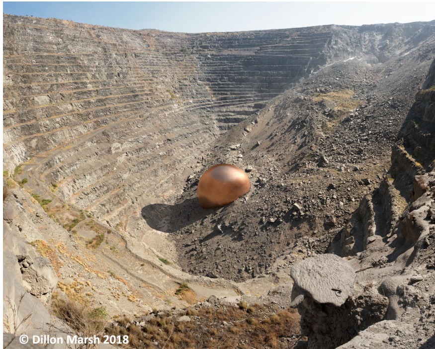
FIGURE 1.1: Visualisation of the volume of copper extracted from a typical open-pit mine. This example is the Palabora Mine in South Africa and the copper ball represents the 4.1 million tons of copper that was extracted. Modified from Marsh (2018).
