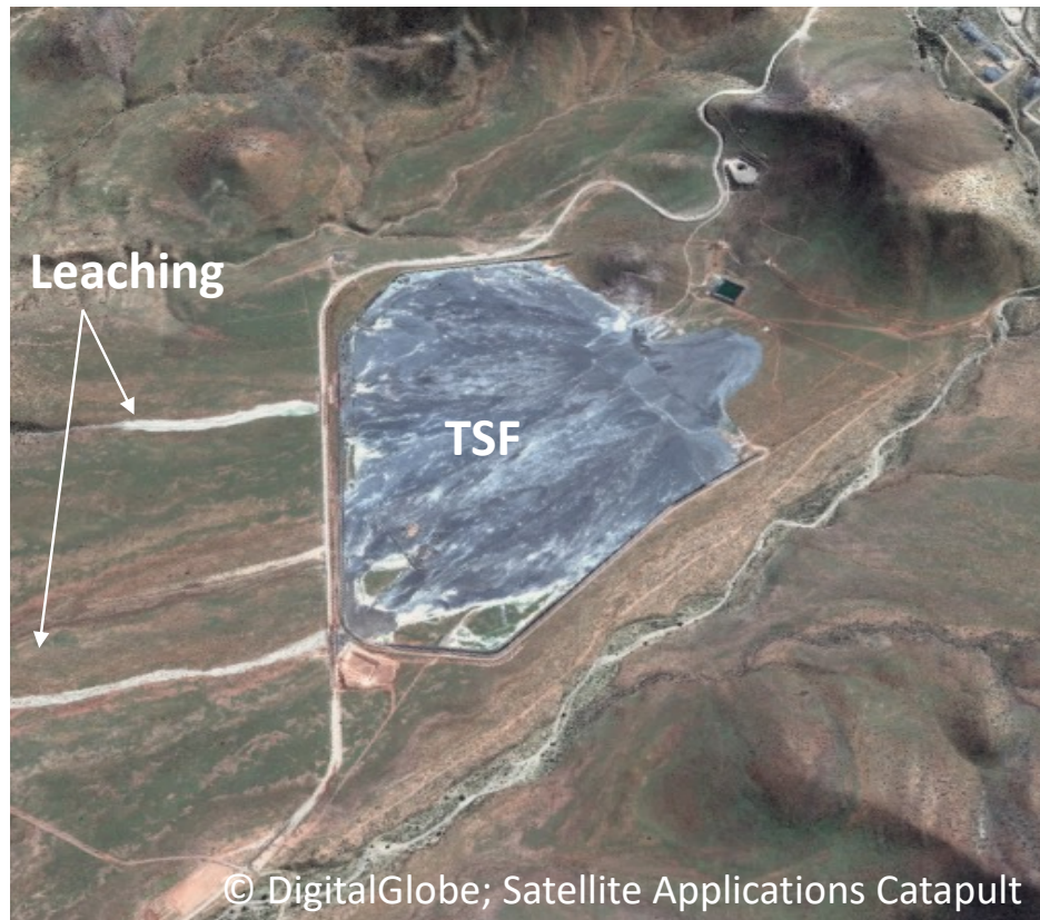
FIGURE 1.4: Tailings material leaching from a TSF in Chile. © DigitalGlobe © Satellite Applications Catapult
