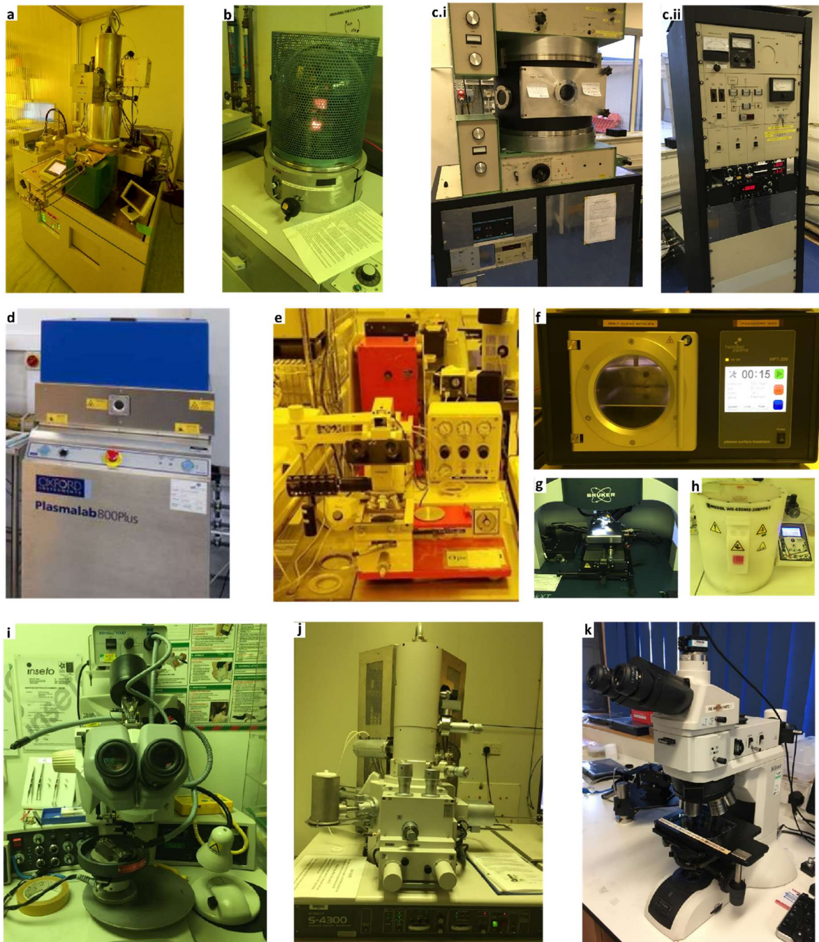
Fig. A. Fabrication and characterisation equipment. a , Electron beam lithography tool (JEOL JBX-5500ZC). b , Thermal evaporator (Edwards 306). c , Sputtering tool chamber ( i ) and control system ( ii ) (Nordiko). d , Reactive-ion etching (Plasmalab 80Plus). e , Mask aligner (Karl Suss MJB 3). f , Plasma cleaning tool (Henniker Plasma HPT-200). g , Profilometer (DektakXT Bruker). h , Spincoater. i , Wire bonder (K&S 4524 Manual Ball Bonder) j , Scanning electron microscope (Hitachi S-4300). k , Optical microscope (Nikon Eclipse LV100 ND).
