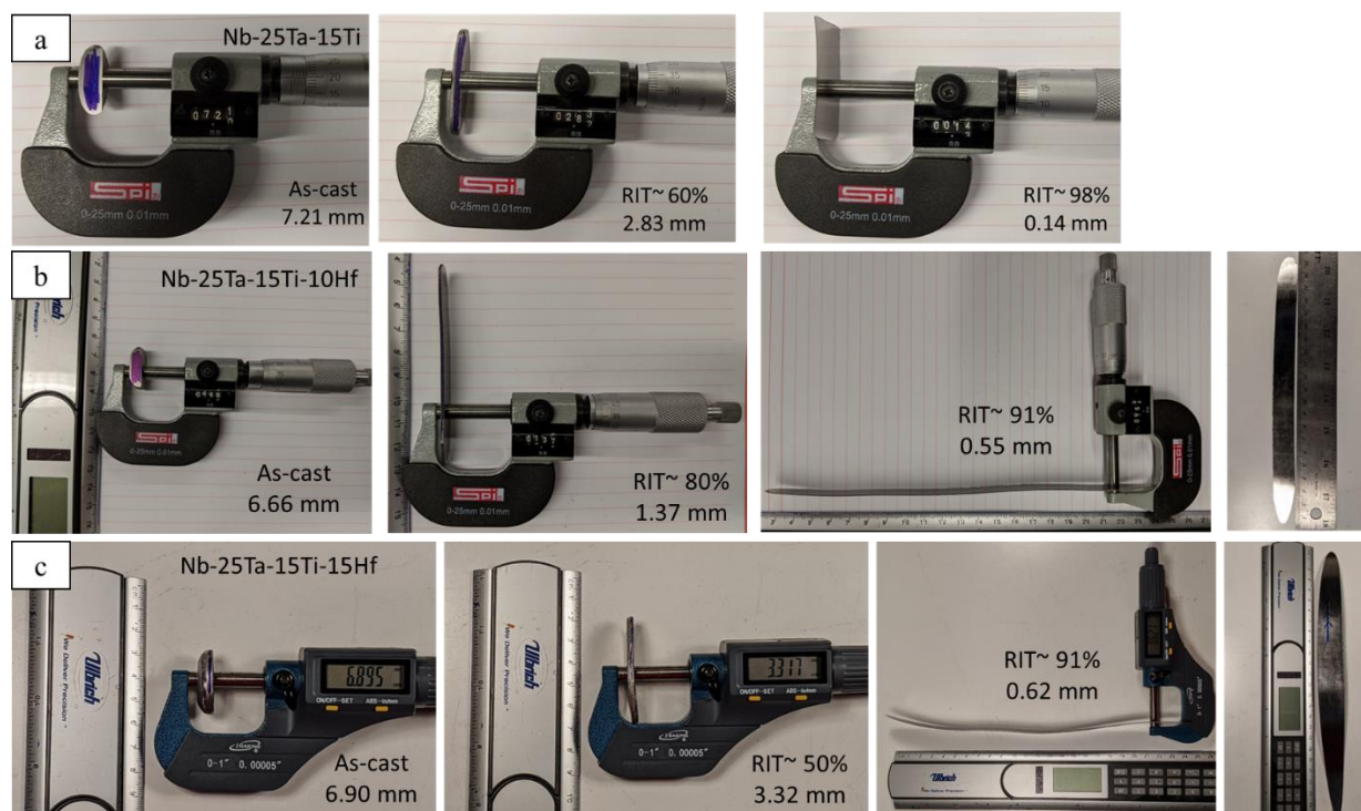
Fig. S2. Images for cold rolled Nb-25Ta-15Ti-based RHEAs from the as-cast state to a reduction in thickness (RIT) over 90%, showing high processability at room temperature. (a) Nb-25Ta-15Ti matrix; (b) Nb-25Ta-15Ti-10Hf RHEA; (c) Nb-25Ta-15Ti-15Hf RHEA.
