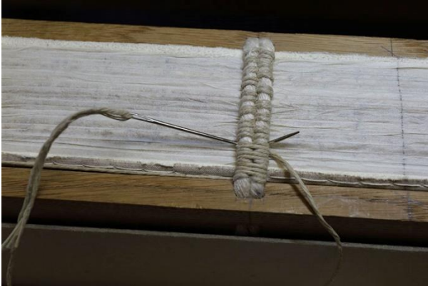
Winchester, Winchester Cathedral MS. 17, Volume II.ii, pack sewing after the boards have been laced on.
