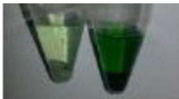
Figure E12. Good quality Cu(I) is shown on the left as a light green to yellow solution. Poor quality Cu(I) insufficient for the reaction is shown on the right (dark green).
