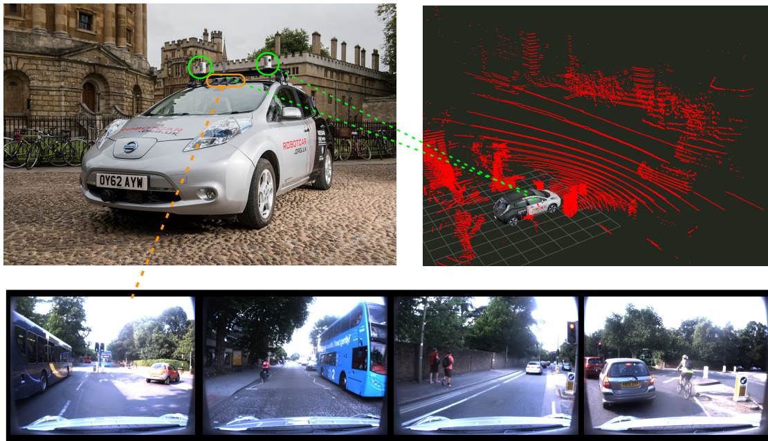
Figure 5.8: We collect data using a NISSAN LEAF vehicle equipped with two Velodyne HDL64E lasers located on either side of the roof (green), as well as a stereo Bumblebee3 camera facing forward (orange). The lasers provide a 360 degree view of the environment around the vehicle, and the stereo images are fed to a visual odometry system to produce ego-motion estimates. We show a selection of forward camera views from the Oxford route driven.
