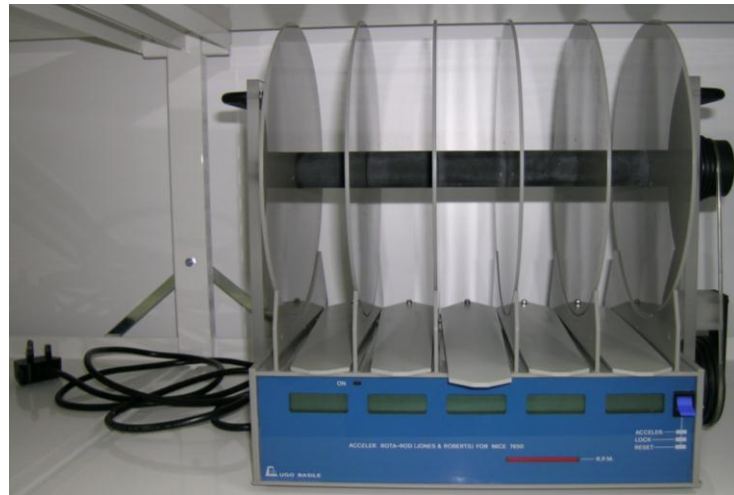
Figure 2.8: Rotarod used for testing Tardbp ENU mutant mice The animals walk on the rolling drum and when falling, the time is automatically recorded.
