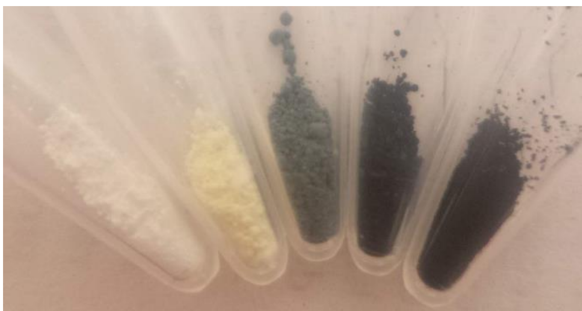
Figure 2.1 A photographic image of N-doped P25 TiO 2 materials. From left to right: pristine P25, N-P25-550, N-P25-600, N-P25-620, and N-P25-660.
