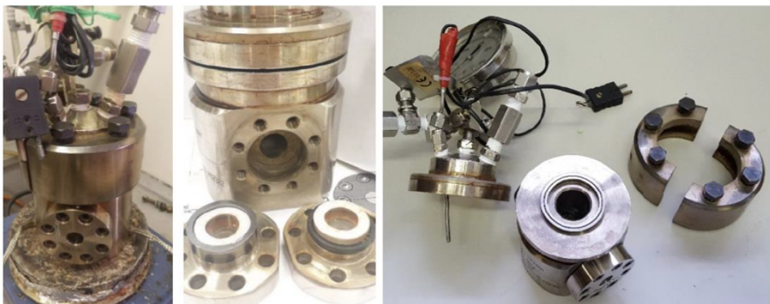
Figure 2.13 Photocatalytic batch reactor for the POWS reaction at elevated temperatures used in this thesis.
