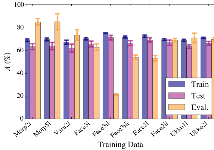
Figure 5: The CNN was trained on 3565 powersweeps from nine of the feed-line datasets, and using those powersweeps as m_t (Train), 180 unseen powersweeps from the same feed-lines as m_t (Test), and all of the powersweeps from the remaining feed-line dataset as m_t (Evaluation), the accuracy parameter A was evaluated from the CNN's predictions ( m_e ). This process was repeated for each of the ten feed-line datasets in turn. When Ukko2 was used as the evaluation dataset, the classifications from first of the four MI operators were used, m_t = MI_A . Each time the CNN was trained for 800 steps of 50 batches. These measurements were repeated ten times and the errorbars are one standard deviation from the mean of the accuracies achieved. The evaluation accuracy parameter achieved with Ukko2 indicates that that dataset is fairly representative of all feed-line datasets.
