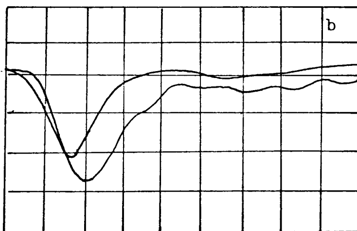
b) CURRENT RECORDED AT THE REAR COLLECTOR C_R AMPLITUDE SCALE - 15 mA/cm. TIME - 40 nsec/cm.
