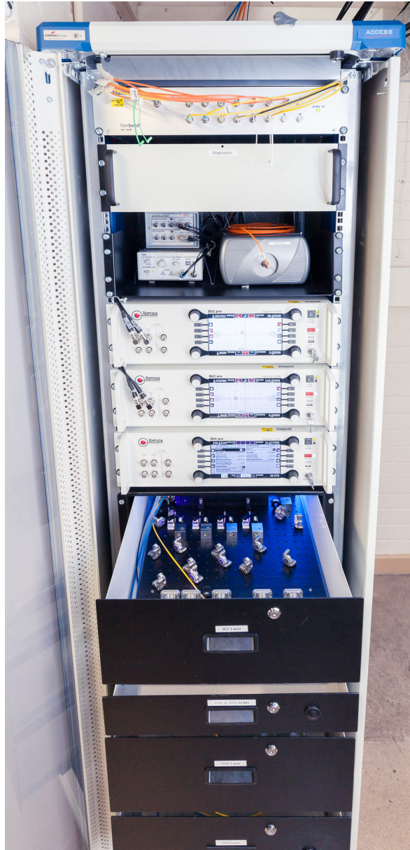
Figure 4.6: Photograph of the 19" rack containing the strontium lasers. Three lasers and their controllers are housed below a laser frequency and spectral diagnostic system. In each drawer, light is split into multiple channels for frequency locking, diagnostics and for the experiment. A neighbouring rack houses AOMs for pulse and frequency control, with reference cavities nearby.
