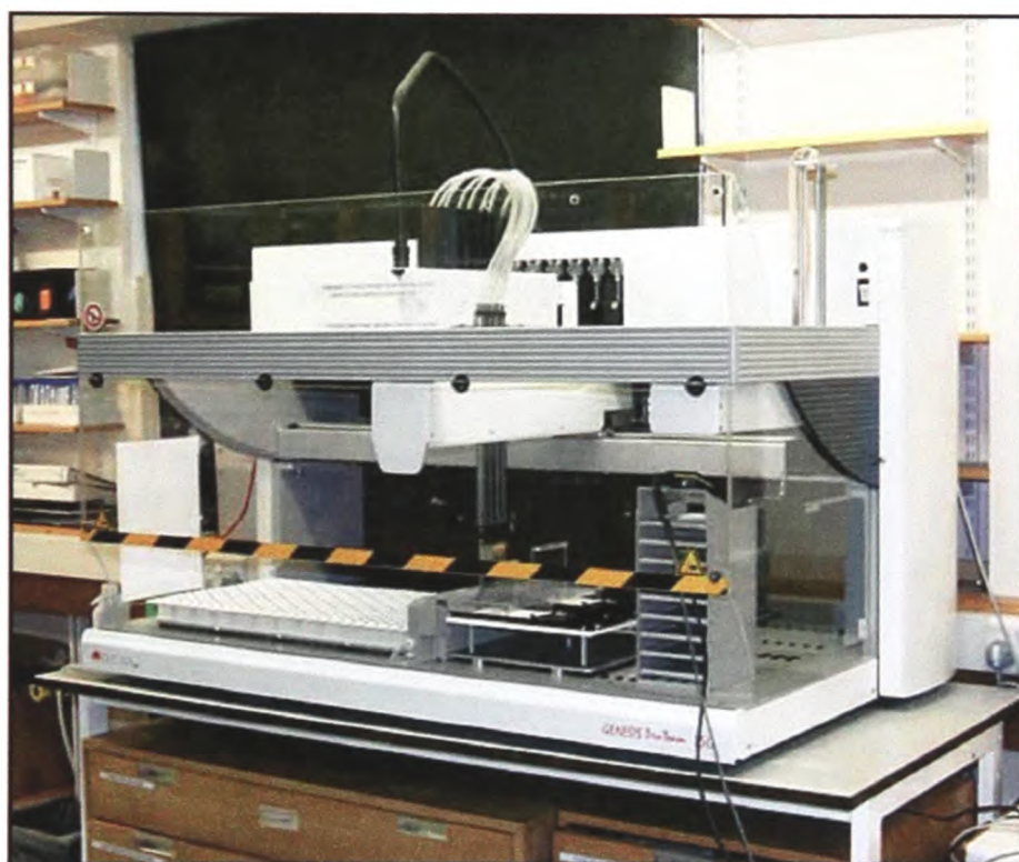
Fig 59. The Tecan Genesis 150 robot used for the preparation of the crystal screens.
