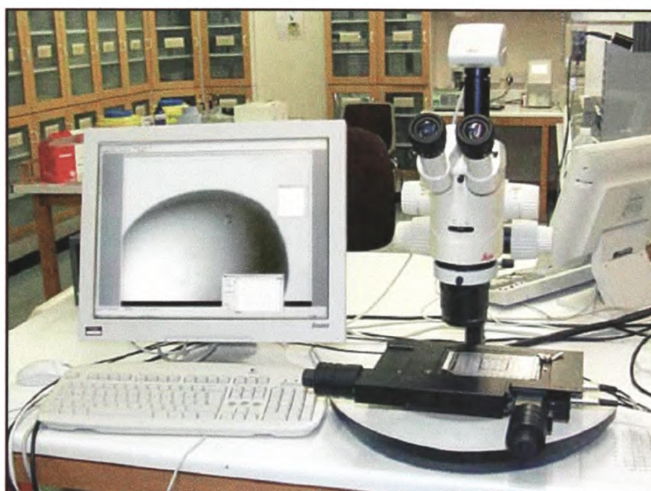
Fig 60. The Leica MZ16 microscope system used for the recording of images of selected drops during the crystal screen trials.
