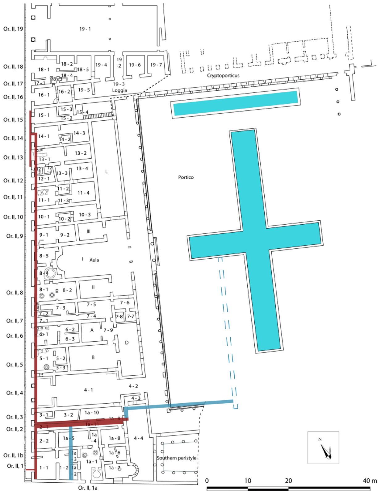
Figure 2.10. The palaestra , Insula Orientalis II and the Cardo V sewer. Red lines indicate the main N-S and E-W branches of the sewer, blue lines indicate later additions. Dashed line is the channel that drained the pool (adapted from pl. V, Monteix 2010). (Permission to reproduce plan granted by N. Monteix)
