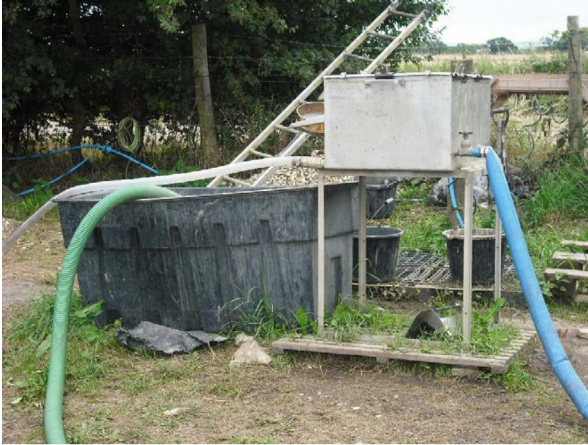
Figure 1.3. A machine assisted flotation device. Water is pumped into the flotation tank until it overflows and water, along with the material that floats, is washed across the sieve (Fig. 1.4). (Permission to reproduce photograph granted by Lisa Lodwick, Silchester Town Life project)
