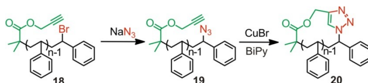
Figure 1.18. Synthesis of cyclic poly(styrene) via atom transfer radical polymerization followed by a “click-coupling by Laurent and Grayson. 81 BiPy=2,2'-bipyridyl.
