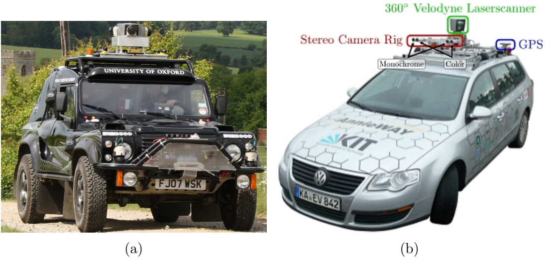
Figure 3.3: The platforms used to collect our real world VO Test datasets. (a) is the Mobile Robotics Group Wildcat vehicle, which is based on the Bowler Wildcat. (b) is the VW Passat used to collect the Kitti sequences. Image from [38].
