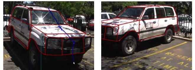
Figure 9: User interaction identifying location of mirror plane (left, sketched mirror line in blue). Model after mirroring showing match with original video (right).
