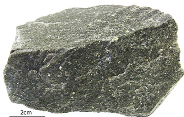
Figure 3.21: Hand specimen photograph of sulphide-bearing, barren Huni Sandstone from Damang.
