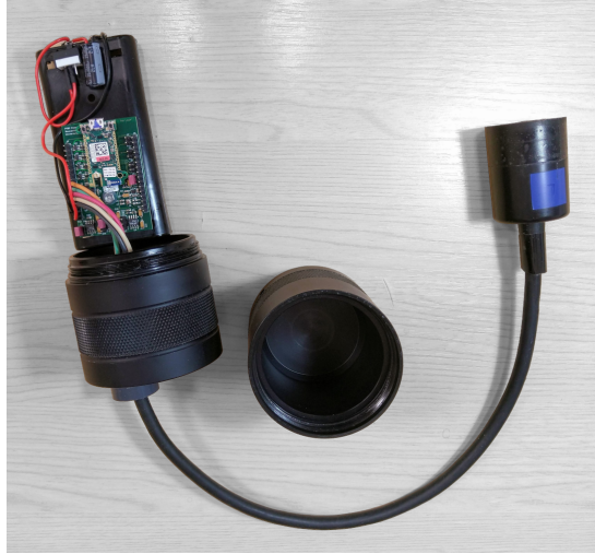
Figure 2: USMART Sensor Node showing the electronics and battery pack within the canister.
