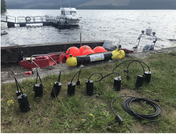
(a) ecoSUBm5 AUV alongside 8 smart sensor nodes (foreground); preliminary tests of the system in July 2021.
