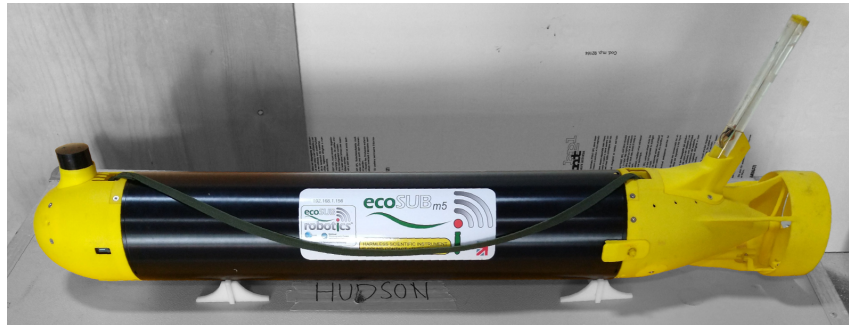
Figure 3: The ecoSUBm5, a micro AUV used in the HUDSON system for underwater data harvesting and navigation tasks.
