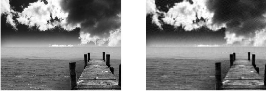
Figure 6.2: Original 768 \times 1024 image with full rank (left); Original image truncated to rank 40 (right).
