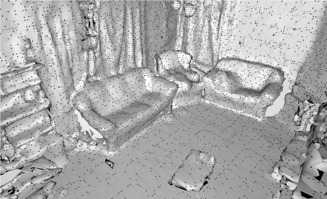
Figure 2.3: Example of HoloLens’ spatial mapping capture in a typical living room. The headset uses multiple depth perception cameras to continuously scan its environment and build a 3D model of its surrounding world. This allows precise indoor localization of the device and ensures that holograms remain statically positioned in space. A mixed-reality view of the same room is shown in Figure 2.4.
