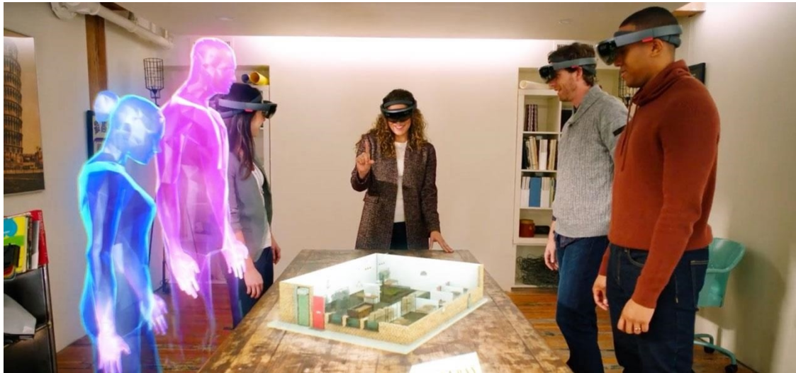
Figure 1.1: Example of a shared mixed reality experience. Some of the participants wearing Microsoft HoloLens are co-located, while some are virtually present. As a result of sharing the common anchor in the physical space, all of the co-located participants can interact with the object at precisely the same location. Source: [14]
