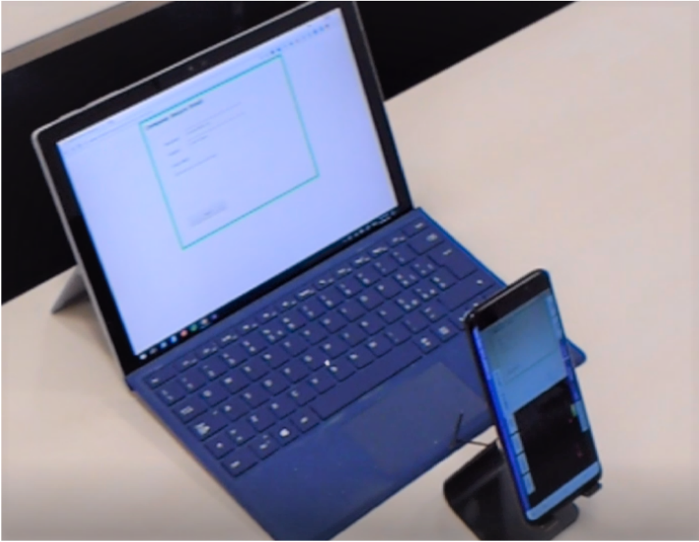
Figure 6.7: Experimental setup. The mobile device is positioned on a simple stand between the user and the client’s screen.
