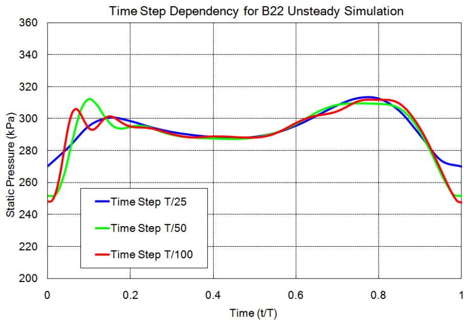
Figure 5.5: Time-step dependency study for unsteady B22 rotor suction surface crown pressure monitor
