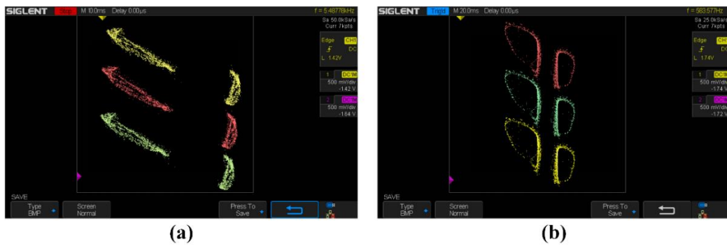
Fig. 17. Phase trajectories with different settings of offset boosting values: (a) MHM1, (b) MHM2.
