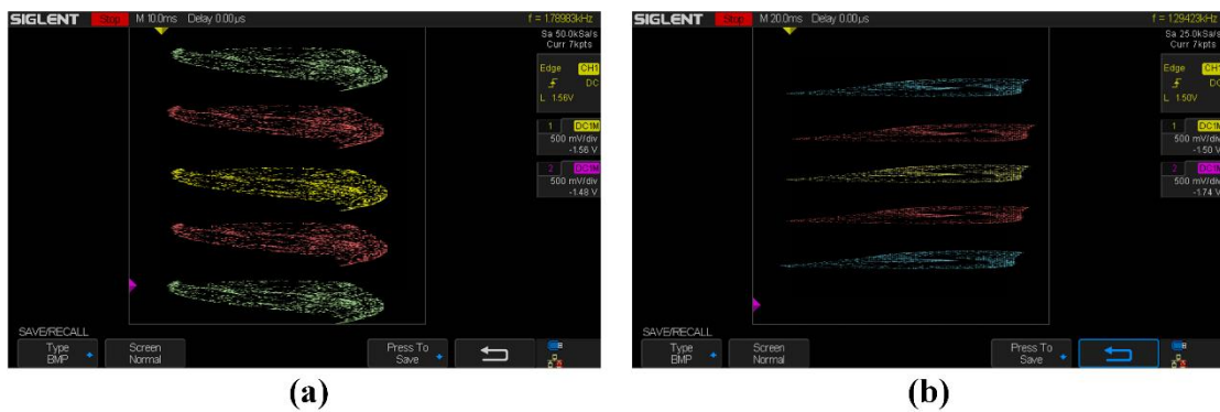
Fig. 19. Discrete sequences in the chaotic maps MHM5 and MHM6 with different initial values of y(0) : (a) MHM5, (b) MHM6.
