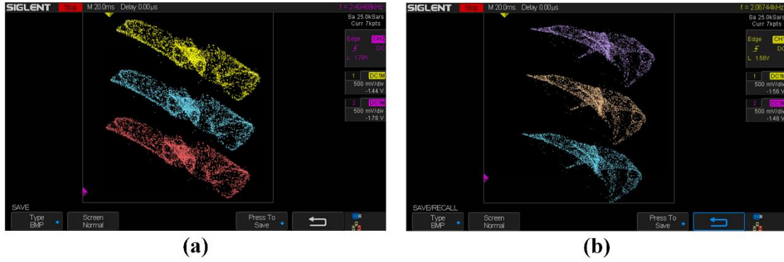
Fig. 18. Discrete sequences in the chaotic maps MHM3 and MHM4 with different initial values of y(0) : (a) MHM3, (b) MHM4.
