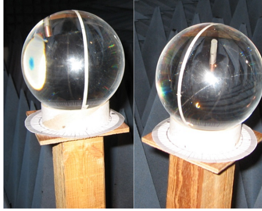
Figure 4.22: Cast P.M.M.A. sphere having a radius of 6 cm with PEC eccentric inclusion.
