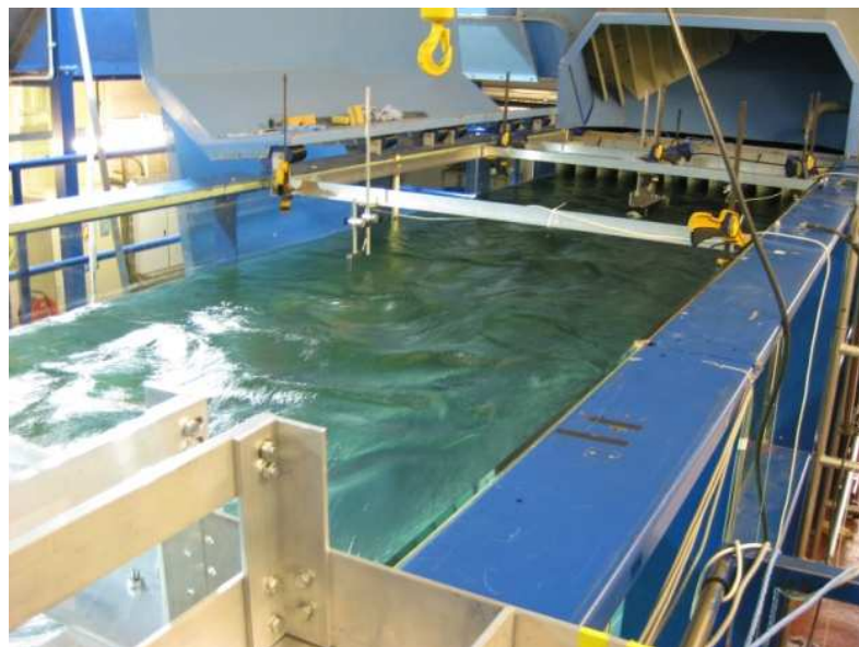
Figure 4.1 – Photograph looking downstream the unobstructed CWWC tank, with a flow depth of 1m
