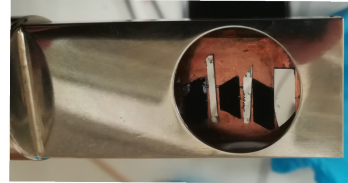
Figure 4.3: Pictures of (a) cold finger, (b) sample holder for quartz discs, and (c) sample holder for wafer pieces with a silver heat shield. To distinguish the various samples (black), thin strips of wafer (shiny), emitting at a different wavelength than the samples, are used as dividers.
