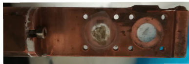
Figure 4.3: Pictures of (a) cold finger, (b) sample holder for quartz discs, and (c) sample holder for wafer pieces with a silver heat shield. To distinguish the various samples (black), thin strips of wafer (shiny), emitting at a different wavelength than the samples, are used as dividers.
