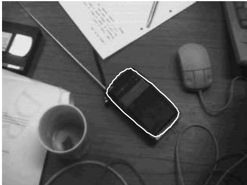
Figure 1.1: A snake in a locally minimum energy configuration. An example of a snake which has been allowed to ‘relax’ into a configuration with locally minimum energy on a static image. The white line shows the snake, a closed quadratic B-spline, attracted to the high-contrast areas at the edges of the radio.
