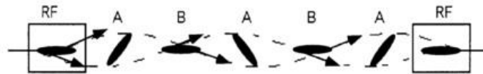
Figure 1.7: An electron bunch is vertically tilted correlated to longitudinal motion by E110 mode using two rf cavities. The longitudinal bunch length is temporary shorter during vertical orientation between two cavity and emits the CSR accordingly [26].
