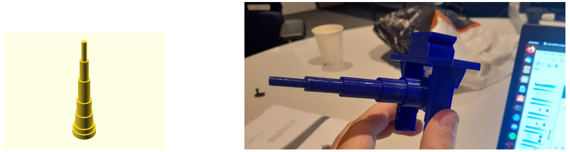
Figure 5.11: PLA S2 visualised in CAD (left) and photograph of 3D printed system set in C-Robot holder (right).
