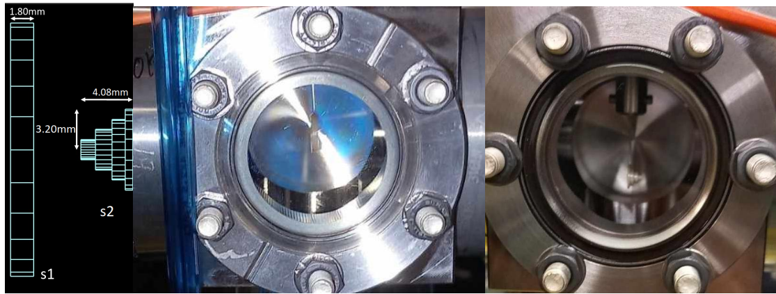
Figure 5.19: Schematic of first vacuum dual-scattering system components at CLEAR (left), camera images of S1 (middle) and S2 (right) installed in beampipe vacuum chambers.
