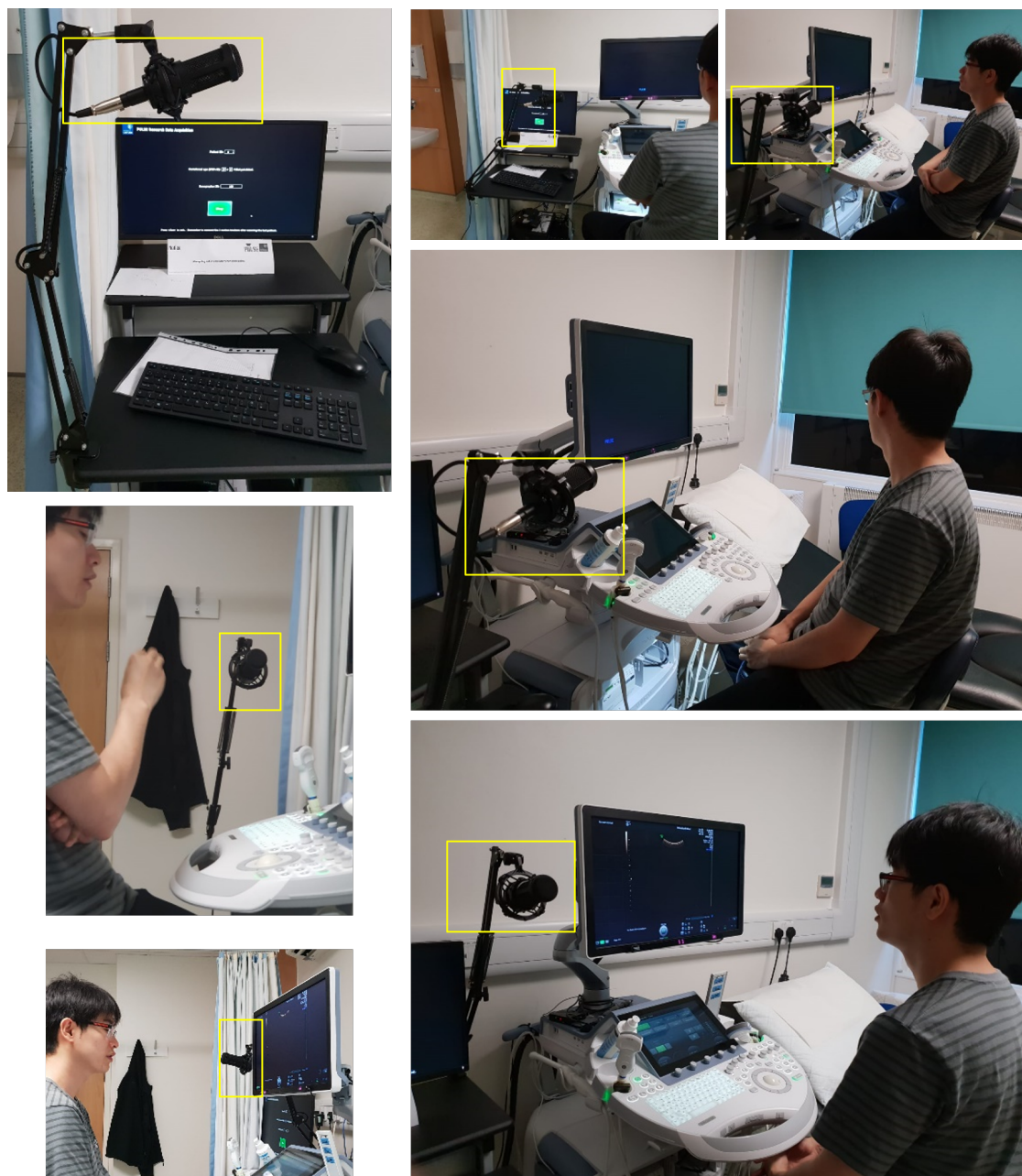
Figure 3.11: How the Audio Technica AT2035 microphone could be installed in the scan room is shown.
