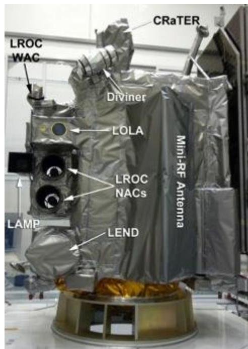
Figure 11: Photograph of NASA's Lunar Reconnaissance Orbiter, with all individual instruments labelled. Taken from Chin et al. (2007).
