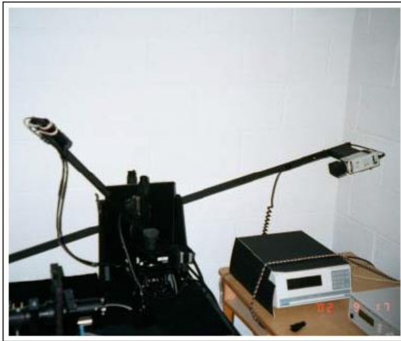
Figure 30: Image of BUG. The longer arm (two meters long) on the right holds the silicon detector. The shorter arm on the left terminates with a fibre-optic lens assembly that puts a near-collimated beam on the sample. Taken from (Johnson & Shepard 2009).
