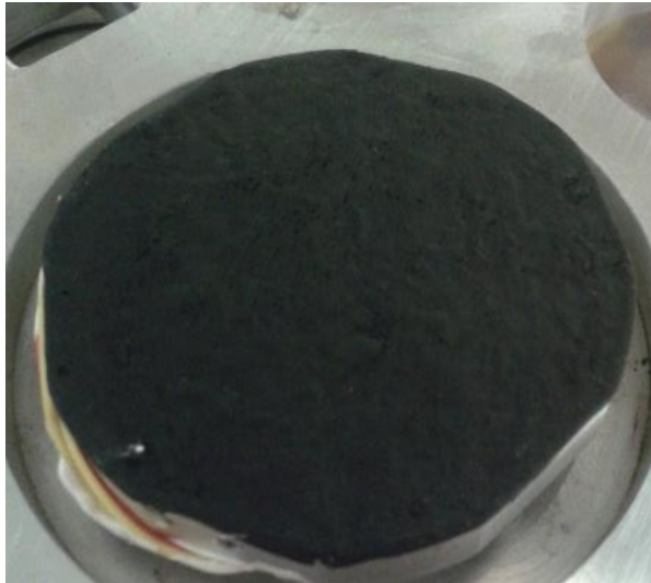
Figure 79: Roughly painted Nextel Velvet black aluminium target 50 mm in diameter.
