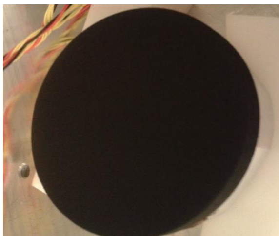
Figure 69: Nextel black painted aluminium target 50 mm in diameter.
